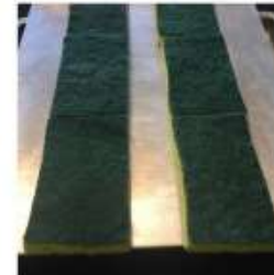
Step 2: Simulate an unhealthy riparian area by laying dry sponges and to end in two rows the length of the cookie sheet, with about 5 cm of space between the rows.
