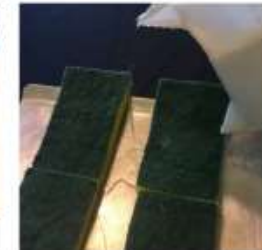
Step 3: Gradually pour a cup of water down the trough between the sponge rows. Some water should seep into the sponges, but most will wash into the pan.
